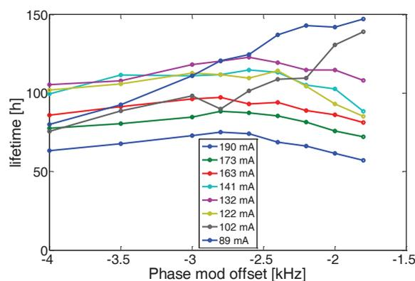
Figure 3: Beam lifetime as function of RF phase modulation offset for a number of beam current.
