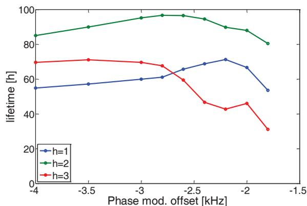
Figure 4: Beam lifetime as function of RF phase modulation offset for the first three synchrotron harmonics.
