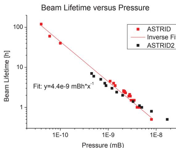
Figure 5: Beam lifetime as function of vacuum pressure.
