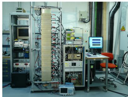
Figure 4: 500 MHz 10 kW unit prototype under long-term test at SOLEIL.
