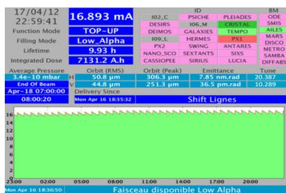
Figure 2: Machine status panel showing successful Top-Up operation in the Low-Alpha mode ( $\alpha/25$ ) achieved in April 2012. The photon beams are delivered to 3 beamlines: AILES, TEMPO and CRISTAL.
