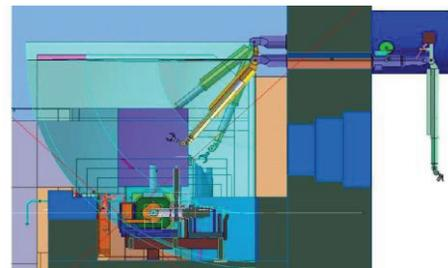
Figure 4: Cross section on the beam line equipment and the interface with the master/slave telemanipulator.
