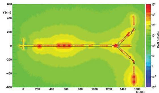
Figure 3: Equivalent dose rate calculation : hot spots on the core beam section in the controlled access area (see Fig. 1). Calculation performed with the MCNPX code and  $^{132}\text{Sn}$  beam (total beam activity is 100 GBq).
