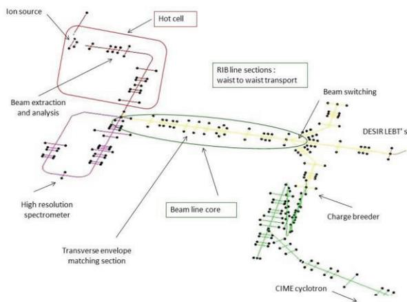
Figure 1: Beam line layout from target and ion source to experiment halls. The core of the beam line connects the hot cell with target and ion source to the secondary beam lines.
