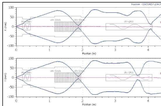
Figure 2: Beam envelopes of the  $^{16}\text{O}^{1+}$  contaminant with settings for the analyzed beam mass 108u,  $\pm 2.25$  mm beam spot,  $80 \pi$  mm.mrad marginal emittance, 1 mA total beam intensity at 60 keV. 99.9 % of the  $^{16}\text{O}^{1+}$  beam is lost after a few meters in front of the ion source inside the hot cell (obtained with the Tracewin code).
