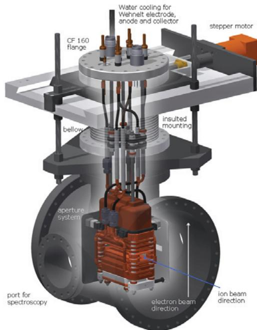
Figure 1: Design of the transversal electron target with manipulator system.
