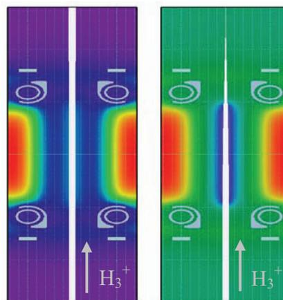
Figure 8:  $H_3^+$  beam with 10 keV through the target. Left: Only electrical fields of the electrodes, no electron beam. Right: Additional superposed fields of electron beam.
