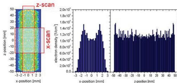
Figure 2: Cross section (left) and averaged electron density profiles for the marked regions (right).
