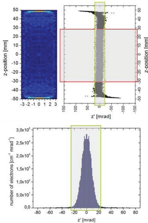
Figure 3: Cross section of the deviation angle in the electron beam and its emittance in ion beam direction. Bottom: Distribution of angle  $z'$ .
