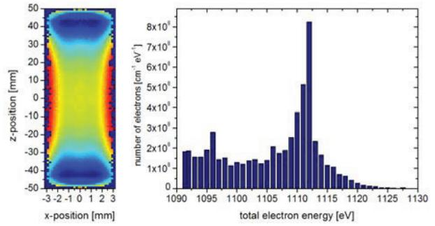
Figure 4: Cross section of the kinetic energy  $T_e$  (left) and the corresponding energy distribution (right).
