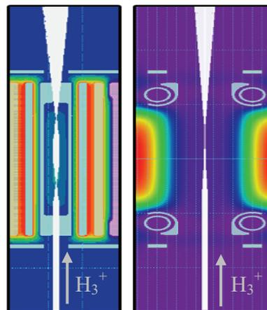
Figure 7:  $H_3^+$  beam with 3 keV propagating through the target. Left: Electron beam direction from left to right side. Right: Electron direction into paper plane.
