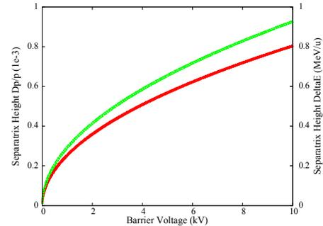
Figure 3: The separatrix height of the barrier bucket as a function of barrier voltage for  $^{238}\text{U}^{92+}$ , 740 MeV/u ion beam. The vertical scale is the barrier height with  $\Delta p/p$  (red line, left scale) and  $\Delta E$  (green line, right scale).
