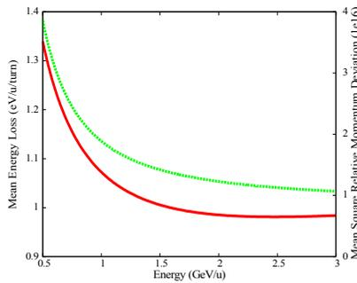
Figure 2: The mean energy loss (red line, left scale) and mean squared relative momentum deviation (green line, right scale) of  $^{238}\text{U}^{92+}$  ion beam in the hydrogen target,  $4e15$  atoms/cm $^2$ .
