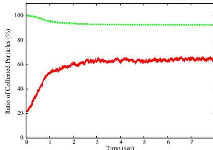
Figure 6: The red line shows the ratio of the particle number within  $-5e-5 < \Delta p/p < 5e-5$  and green line  $-6e-4 < \Delta p/p < 6e-4$ . The barrier voltage is 2 kV.
