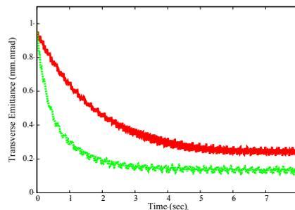
Figure 7: The evolution of transverse emittance. Red: horizontal emittance and Green: vertical emittance.
