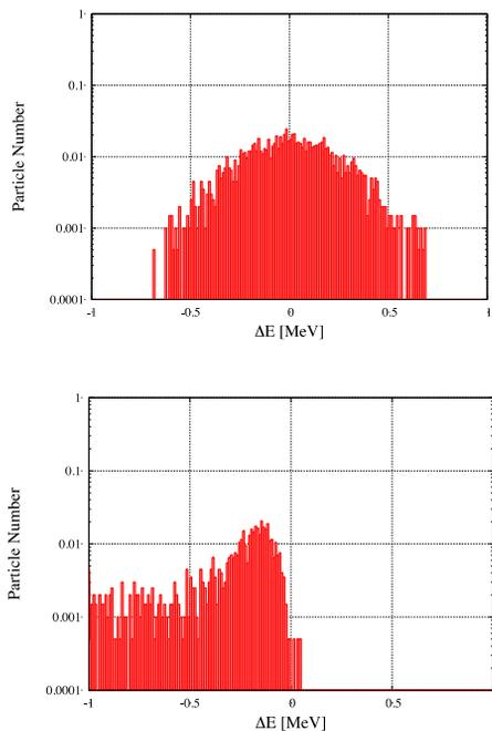
Figure 4: The energy spectra for different time. From the top, time=0 sec and 8.0 sec, respectively without barrier voltage.
