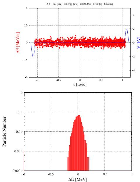
Figure 5: Particle distribution in the longitudinal phase space (top), and the energy spectrum (bottom) after 8 sec cooling. The barrier voltage is 2 kV.
