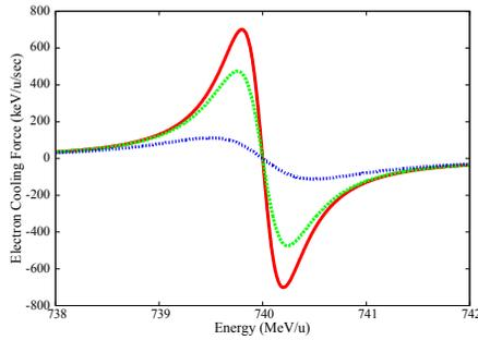
Figure 1: Longitudinal electron cooling force for  $^{238}\text{U}^{92+}$ , 740 MeV/u ion beam as a function of beam energy. The horizontal scale is beam energy and the vertical scale is the longitudinal cooling force. The parameters are transverse emittance, 0.01 (red), 0.1 (green) and 1.0  $\pi$  mm.mrad (blue), respectively.
