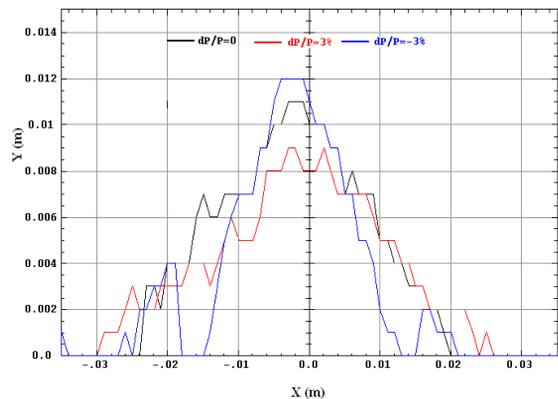
Figure 4: Dynamic aperture with SCW-31. The on/off momentum particles have been tracked 3000 turns through the ring.
