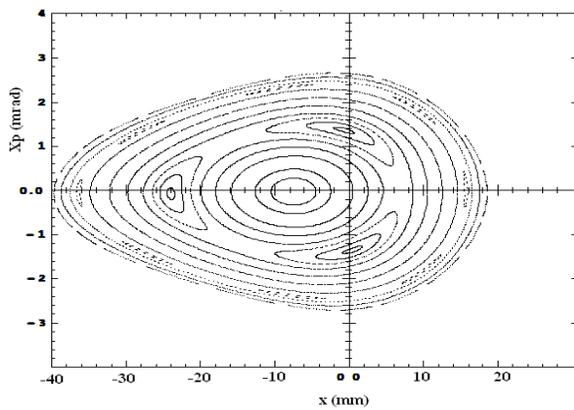
Figure 5: Horizontal phase space for a particle with -3% energy deviations. The SCW-31 is included in the ring.
