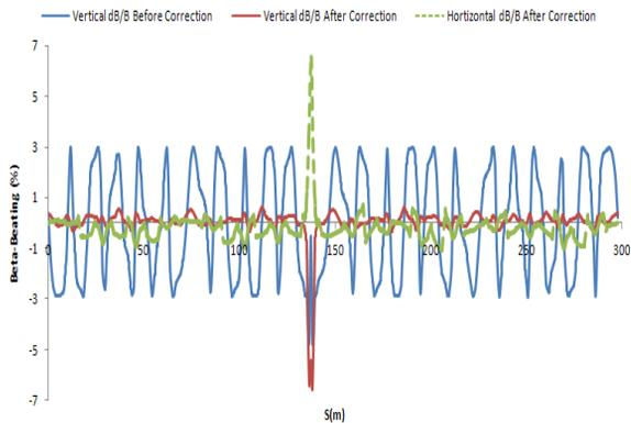
Figure 2: Beta beating ( $\Delta\beta/\beta$ ) along the ring with one SCW-31 in medium straight section before and after correction. The picked point represents beta beating in SCW-31.
