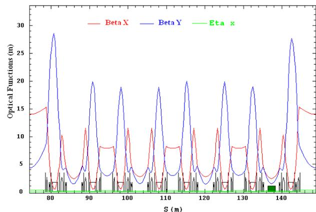
Figure 1: Optical functions in one super period of the ILSF storage ring. The SCW-31 is specified with a green box in a medium straight section.
