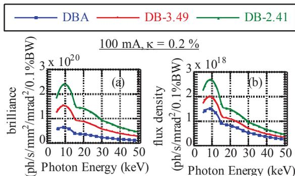
Figure 1: (a) Brilliance and (b) flux density from standard undulator ( $l_u = 32$  mm,  $L = 4.5$  m,  $K_{max} = 2.5$ ) calculated by SPECTRA [3].
