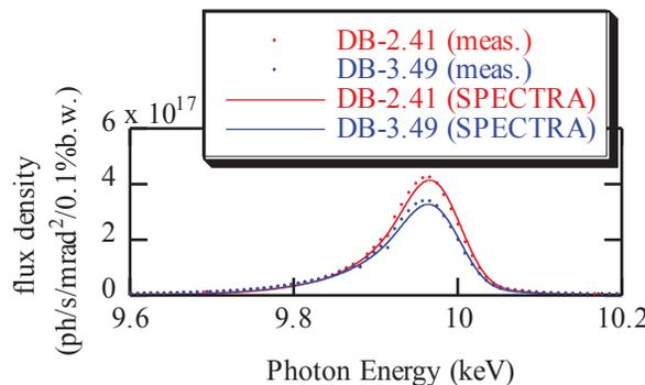
Figure 6: Flux density at the diagnostics beamline II ( $I_u = 76$  mm,  $N = 51$ ,  $K=1.666$ , 3rd harmonic).
