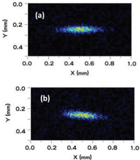
Figure 5: X-ray beam image for (a) DB-3.49 and (b) DB-2.41. The tilt of these images is not absolute and the ambiguity is mainly due to an optical system.
