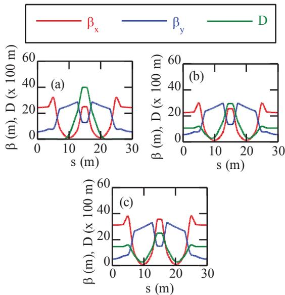
Figure 2: Lattice function of (a) DBA optics, (b) DB-3.49 and (c) DB-2.41:  $\beta$  is the betatron function and  $D$  is the horizontal dispersion.
