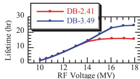
Figure 3: Touschek lifetime vs. RF voltage.
