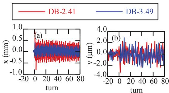
Figure 4: Oscillation of stored beam when bump magnets are tuned on in (a) horizontal and (b) vertical direction.
