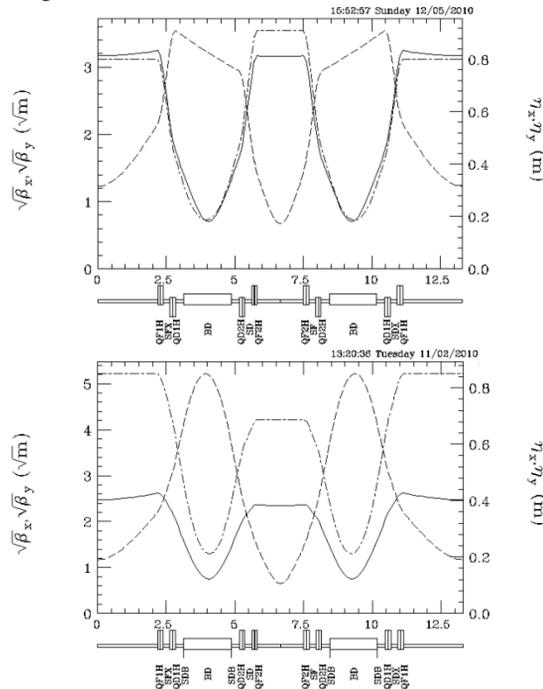
Figure 2: Optics of UVSOR-II (up), and III (down). The betatron functions in the horizontal and vertical plane (solid and dashed line) and the dispersion function (chain line).
