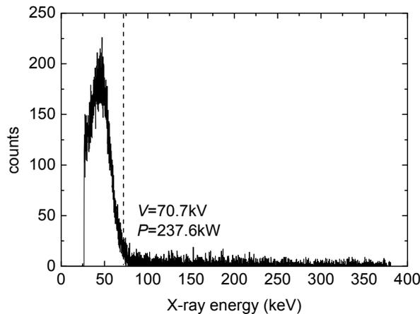
Figure 3: Roentgen spectrum at 237.6kW.
