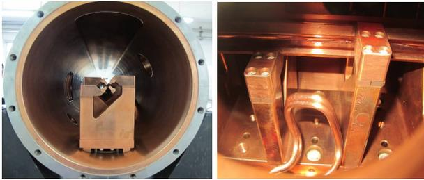
Figure 2: RFQ inner structure (above left), Magnetic coupler (above right).
