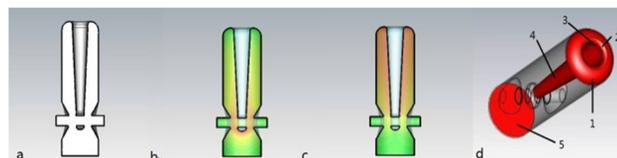
Figure 1: Initial designed QWR model. (a is prototype, b is the electric distribution, c is the magnetic distribution and d is the five regions (red areas) to be checked.)
