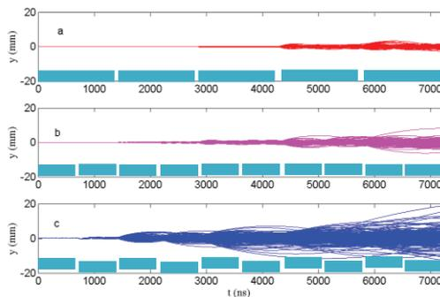
Figure 3: The oscillation amplitude of ions with respect to the circulating time in SSRF storage ring. a) 1 bunch train with 700 bunches followed by 20 empty gap, b) 2 bunch trains with 350 bunches each, separated by 10 empty gap and c) 2 bunch trains with 350 bunches each, separated by 10 empty gap, run at different closed orbit depart with distance in between about 200 $\mu\text{m}$ .
