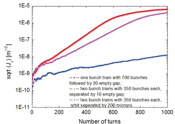
Figure 4: Growth of maximum oscillation amplitude for cases as for Fig. 3.
