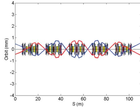
Figure 1: Sketch of the closed orbits for Two Twisted Beam operation mode in SSRF storage ring (a quarter of the full ring lattice is shown here).
