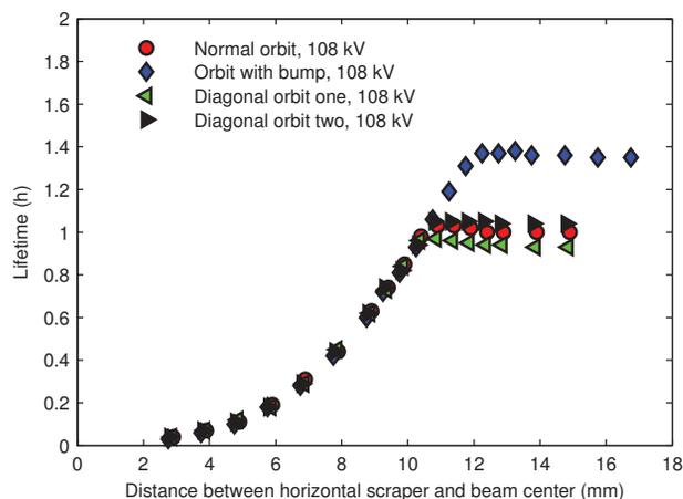
Figure 3: Horizontal scraper measurements for the four different orbits from Fig. 2. The error of the measured lifetime is estimated to be smaller than  $\pm 0.3\%$ . The uncertainty in the location of the beam center is estimated to be  $\pm 0.2$  mm.
