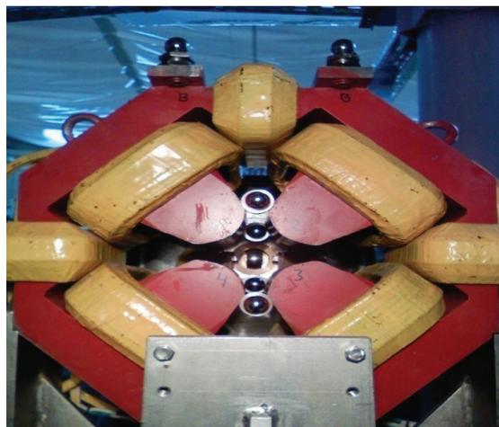
Figure 5: Quadrupole lens during fiducialization procedure.
