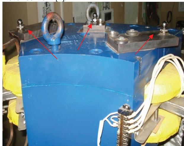
Figure 3: Target balls of the transportation channel dipole magnets.
