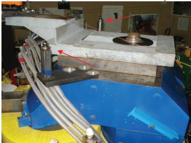
Figure 4: Dipole magnet of storage ring (target balls is shown arrows).
