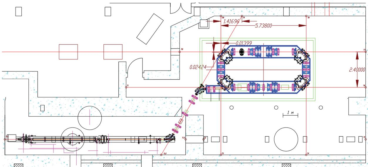
Figure 1: Layout of the NESTOR facility coordinate net.
