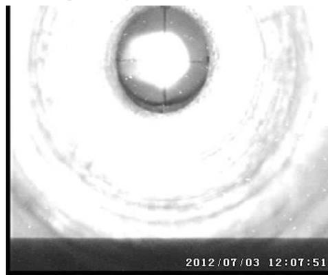
Figure 4: Optimized electron beam sizes at the exit of linear accelerator (RMS sizes: x-direction is about 5 mm, RMS sizes: z-direction is about 5 mm,)
