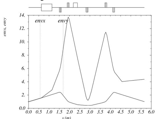
Figure 3: Transverse sizes of the beam along the transport channel in the second stage.  $em_{vx}$ ,  $em_{vy}$  - horizontal and vertical size, respectively.
