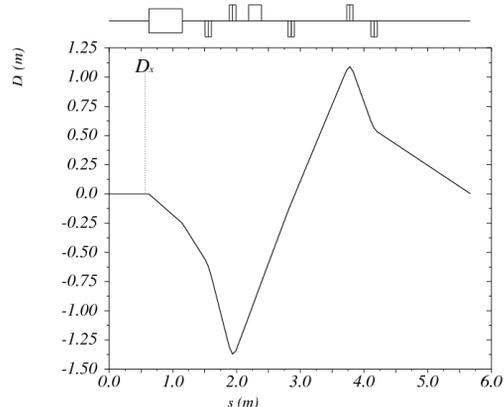
Figure 2: Dispersion function along the transport channel in the second stage.
