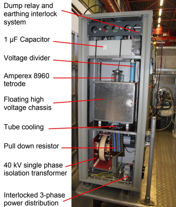
Figure 1: Inside the extraction voltage power supply.
