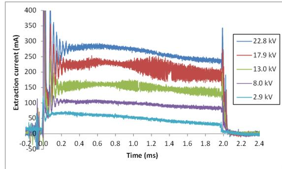
Figure 6: Extraction currents for different extraction voltages at 2 ms 50 Hz extraction from a running ion source.
