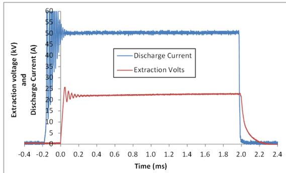
Figure 4: A 23 kV, 2 ms 50 Hz extraction from a 50 A, 2.2 ms, 50 Hz ion source discharge.
