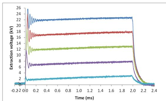
Figure 5: 2 ms 50 Hz extraction voltage pulses of various amplitudes.
