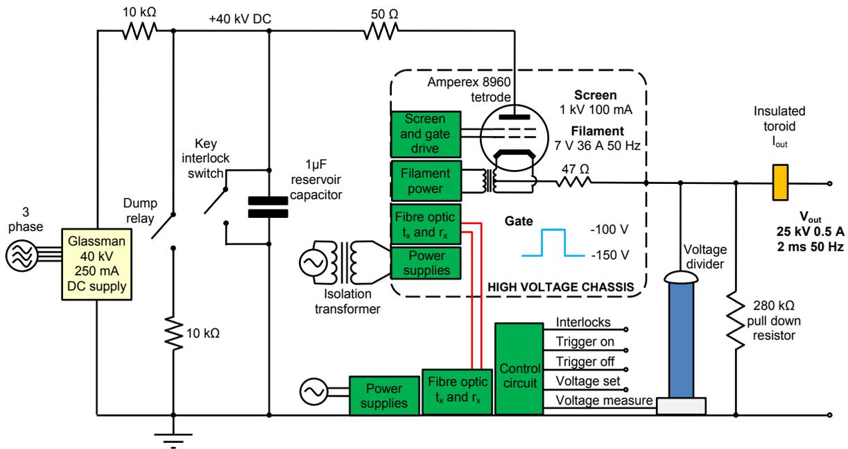
Figure 3: Schematic showing the operation of the pulsed extraction power supply.
