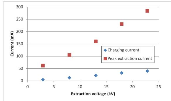
Figure 7: Peak pulsed extraction currents and reservoir capacitor DC charging currents for different extraction voltages at 2 ms 50 Hz.
