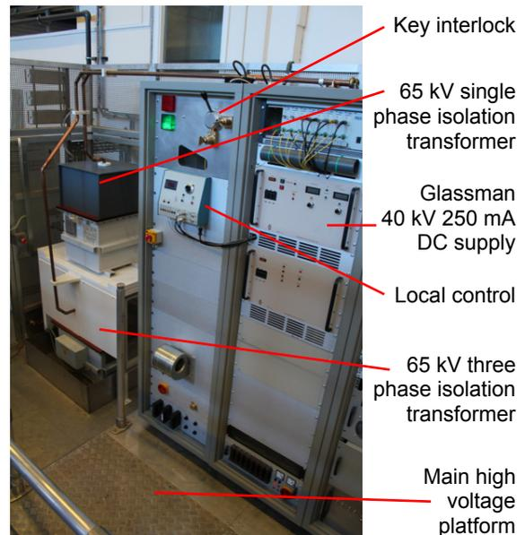
Figure 2: Power supply on the high voltage platform.
