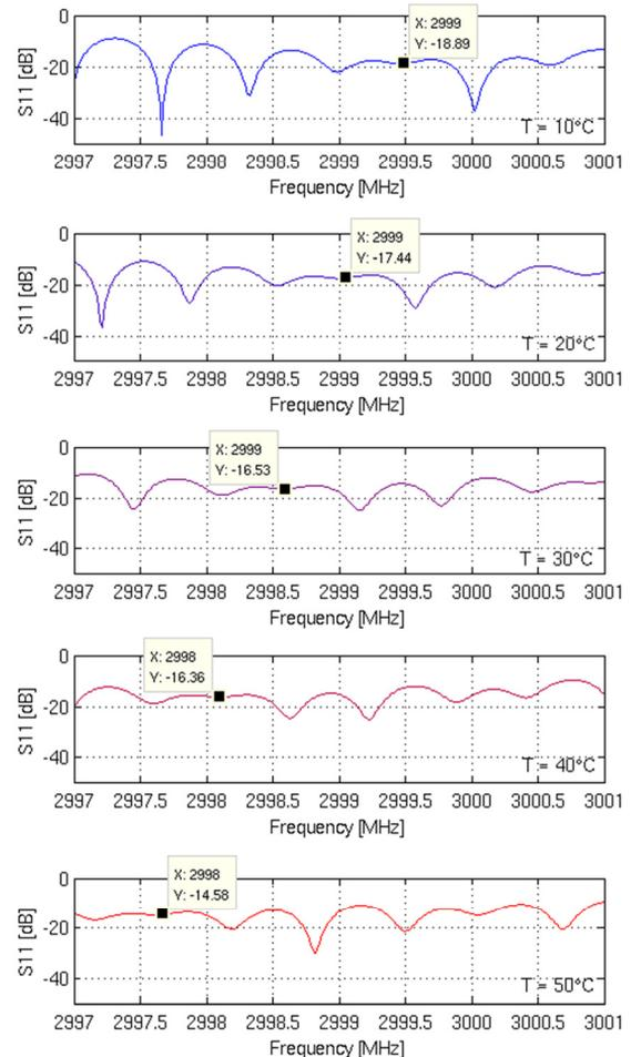
Figure 4: Temperature scan of linac TM<sub>010</sub> modes.
