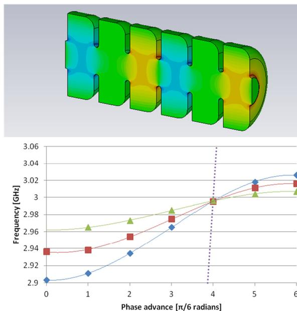
Figure 3: Dispersion curves of first (blue), middle (red) and last (green) cell of Diamond linac accelerating structure.
