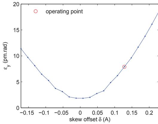
Figure 1:  $\epsilon_y$  as a function of skew quadrupole offset for standard conditions (300 mA, 900 bunches, IDs closed).
