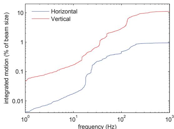
Figure 5: Projected electron beam motion at the centre of a standard straight with fast orbit feedback running. Data plotted as a percentage of electron beam size ( $\epsilon_x = 2.7$  nm.rad,  $\epsilon_y = 8$  pm.rad).
