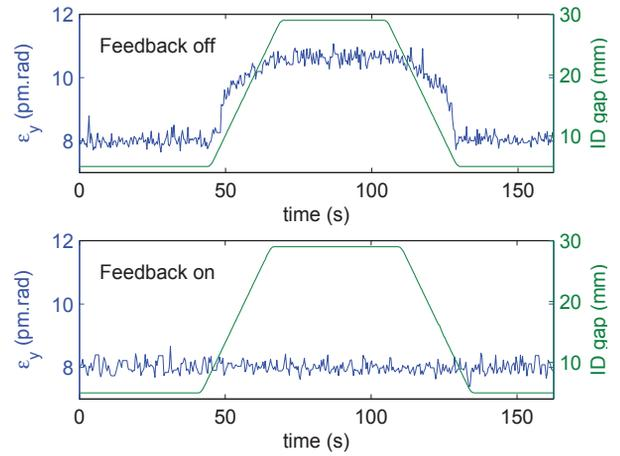
Figure 2:  $\epsilon_y$  variation with I02 gap, with and without vertical emittance feedback ( $f$  and  $\alpha$  set to 0.5).
