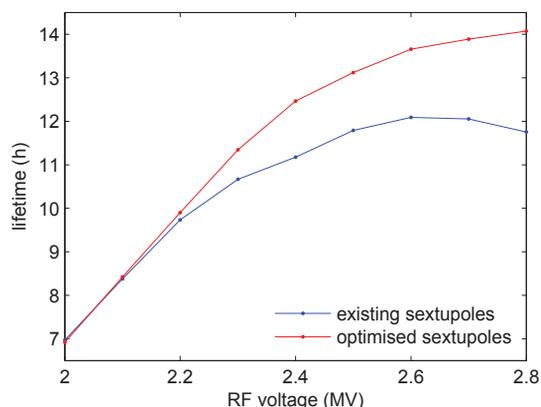
Figure 4: Comparison of lifetime as a function of RF voltage for two sets of sextupoles. Data recorded for standard user conditions (300 mA, 900 bunches,  $\epsilon_y = 8$  pm.rad, IDs closed).
