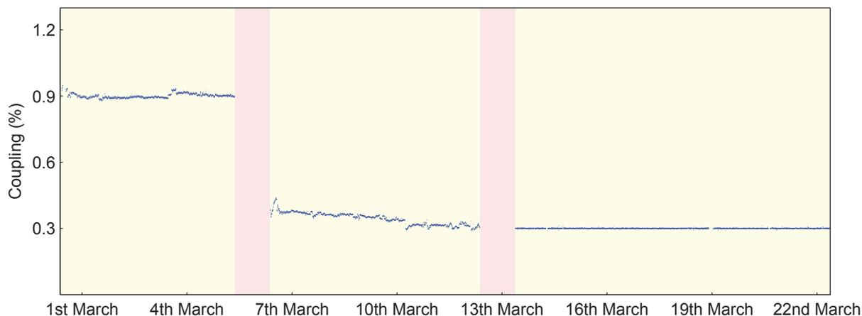
Figure 3: Emittance coupling ratio during three weeks of user operation. The period covers operation at 1% coupling, the switch to 0.3% coupling and 0.3% coupling with feedback enabled. Machine development days are highlighted in red.
