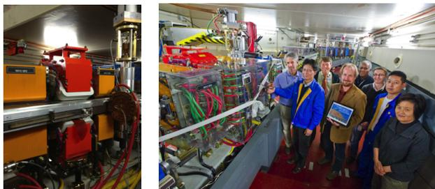
Figure 5: Left: SHD magnet installed between the QF and QD quadrupoles. Right: Ribbon capping celebration after successful installation.
