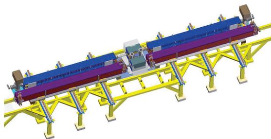
Figure 1: The wiggler switchyard in the middle of the FEL straight section. Electrons travel from the left to the right.
