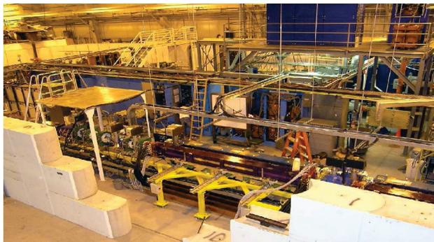
Figure 3: A picture of the completed wiggler switchyard system in June, 2012 before restoring the shielding wall.
