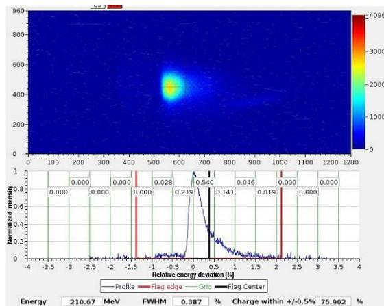
Figure 2: Energy spectrum of 210 MeV 11 nC beam in the MBM mode.
