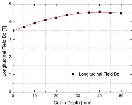
Figure 2: Peak longitudinal field as a function of cut-in cone depth.
