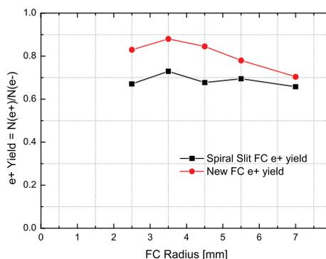
Figure 5: Positron yield as a function of FC radius in the end of capture section. The red and black line represents the new FC and spiral slit FC respectively.
