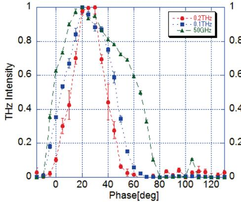
Figure 9: Phase dependence of 0.1 THz with BPF (0.2 THz) (red), 0.1 THz (blue), and 0.05 THz (green).
