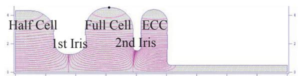
Figure 2: SUPERFISH Drawing of ECC rf gun.
