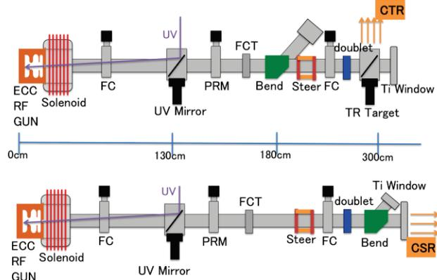
Figure 6: Beamline layouts for CTR (above) and CSR (below).
