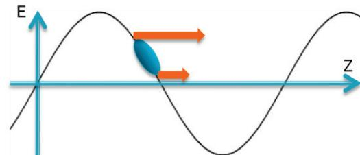
Figure 1: Off-crest rf phase acceleration in ECC.
