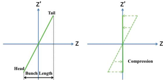
Figure 3: Bunch compression in phase space.
