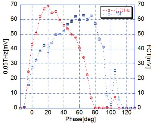
Figure 8: Phase dependence of 0.05 THz CSR.
