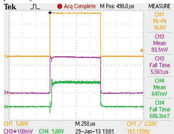
Figure 4: Faraday cup signal in drift I.
