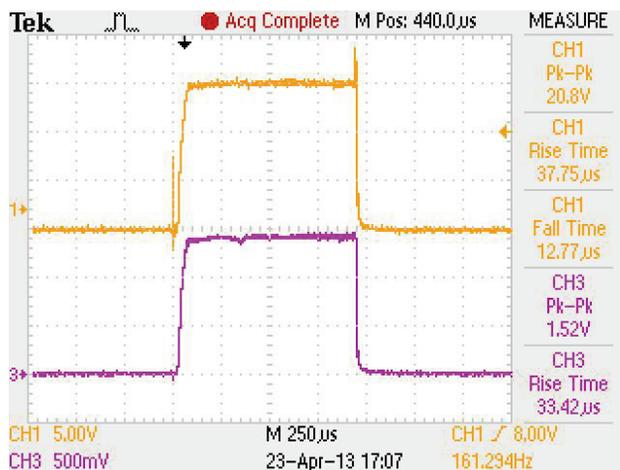
Figure 6: ACCT(CH1) and Slit Cup(CH3) signals.
