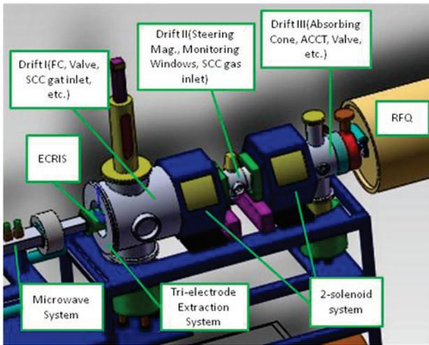
Figure 1: Mechanical review of injector.
