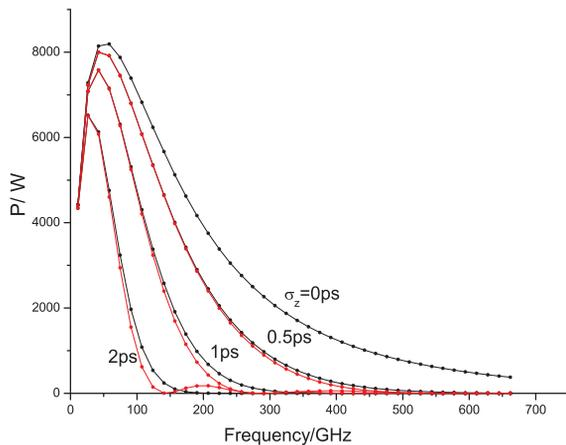
Figure 6: The power of wakefield radiation as a function of frequency, for bunches with different rms length. The black line is for gaussian shape, and the red line is for uniform shape.
