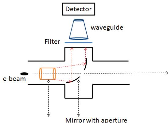
Figure 7: The sketch of measurement setup.
