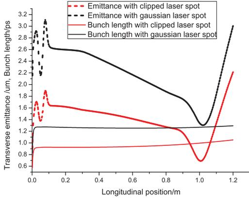
Figure 3: Transverse emittance and rms bunch length vs longitudinal position for different laser spots.
