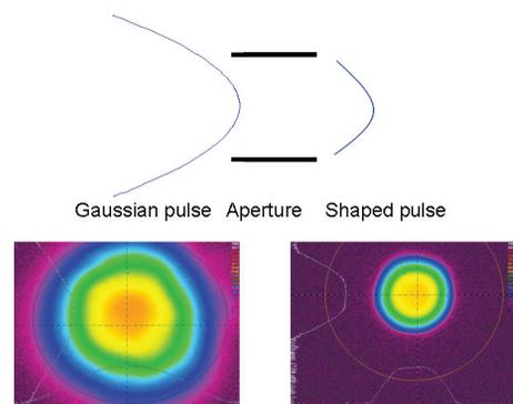
Figure 2: Clipping shaping: sketch and shaping result (UV light).
