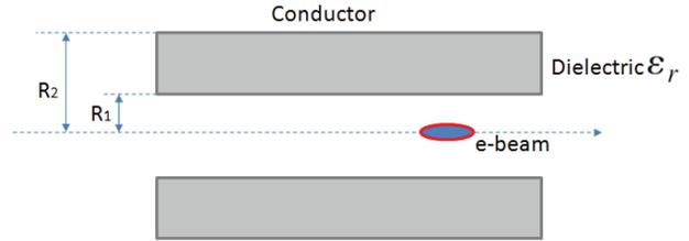
Figure 5: The sectional drawing of a beam-driven cylindrical dielectric-lined waveguide.
