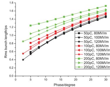
Figure 1: The rms bunch length vs. acceleration phase at different charges and acceleration gradients.
