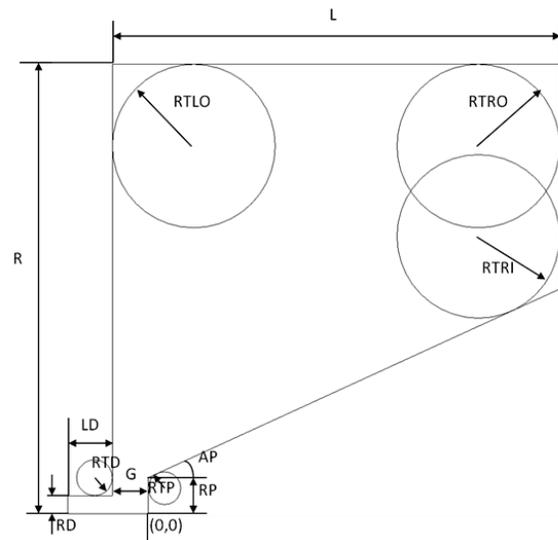
Figure 2: Parameterized dimensions of the gun cavity.
