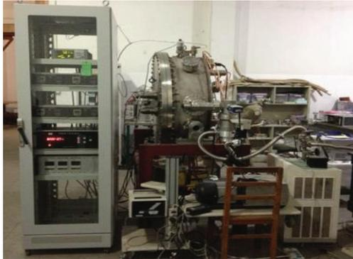
Figure 7: Gun cavity proto-type in test area.
