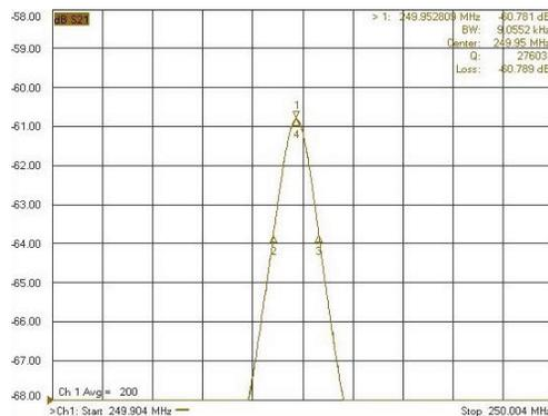
Figure 8: RF measurement of the gun cavity proto-type.
