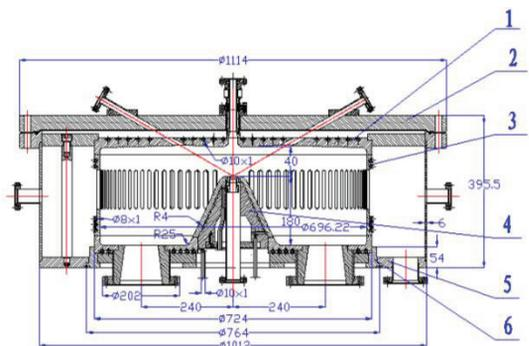
Figure 5: Mechanical design of the gun cavity proto-type.
