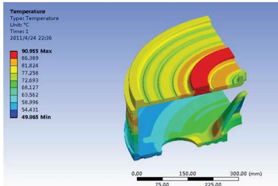
Figure 6: Temperature distribution in the gun cavity.
