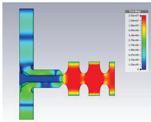
Figure 1: 3D CST calculation of electric field in the front-coupling 2.5 cell cavity (VELA/ALPHA-X gun design).
