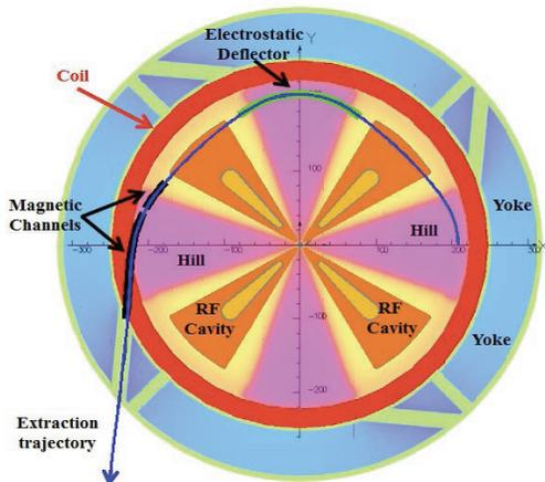
Figure 1: The Injector
