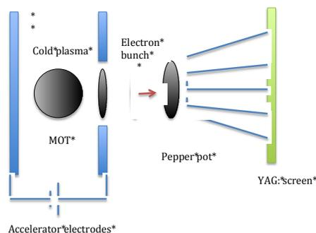
Figure 2: Schematic of the PSI cold electron source with beam extraction and the characterization system.
