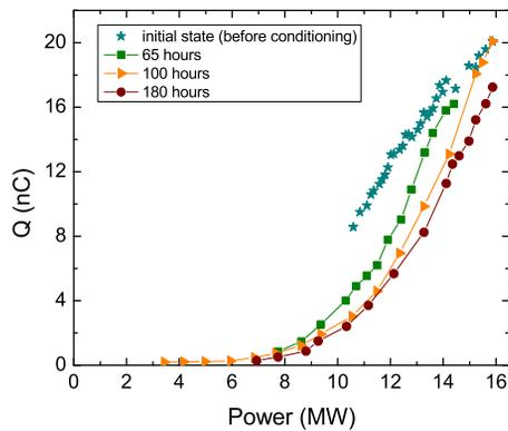
Figure 2: Initial conditioning with Cu cathode. Plot of charge measured with the Faraday cup vs. RF power into the gun. Dark current levels declined from the initial level at the operating point (12 MW) by 50% after conditioning. 12 MW input power provides a max field on the cathode of about 80 MV/m.
