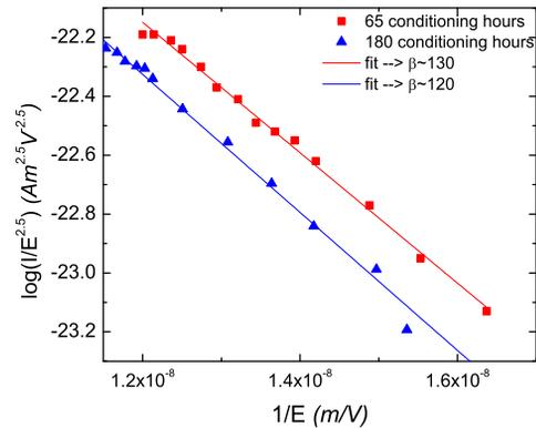
Figure 3: Fowler-Nordheim plots for the Cu cathode at two different points in the conditioning process. The field enhancement factors ( $\beta$ ) derived from the plots indicate that the field enhancement decreased by almost 10% after an additional 115 hours of conditioning.
