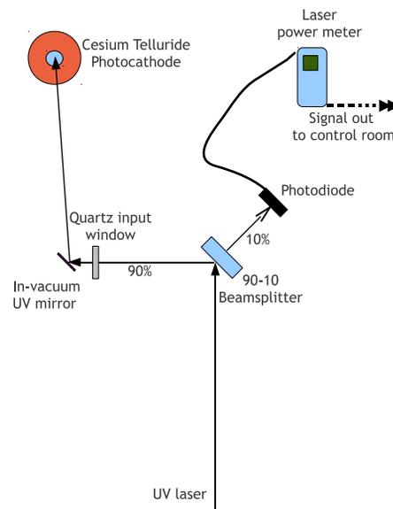
Figure 4: The experimental setup for measuring laser input power for the planned photoemission studies in the gun. The laser power measurement will be correlated with the ICT signal for shot to shot QE measurements.
