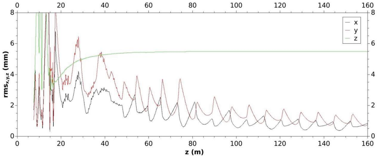
Figure 3: Designed electron beam optics at the SNS superconducting linac for 5 mA electron beam current.
