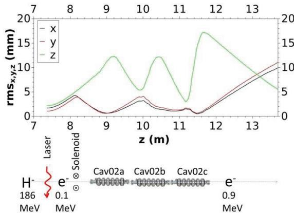
Figure 2. Optimized solution for the electron beam acceleration in the first cryomodule.
