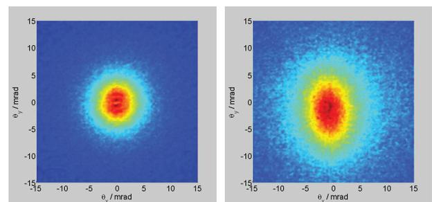
Figure 2: Measurement of the PXR angular distribution for the (220) reflex. Left: beam size  $\sigma_x = 45.7 \mu\text{m}$  and  $\sigma_y = 42.9 \mu\text{m}$ , right:  $\sigma_x = 44.7 \mu\text{m}$  and  $\sigma_y = 796 \mu\text{m}$ .
