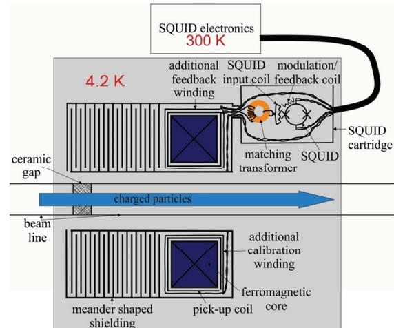
Figure 5: Cross section of the improved SQUID-based CCC for FAIR.
