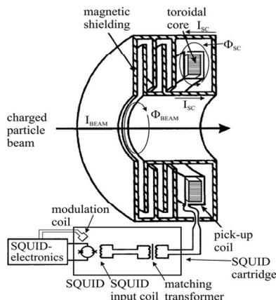
Figure 1: Simplified schematic view of the CCC with magnetic shielding, pick-up coil, and SQUID system.
