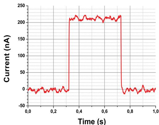
Figure 8: Response of the welded pick-up coil with Nanoperm M-764-01 core connected to the SQUID sensor enclosed into the niobium enclosure to a rectangular current signal of 220 nA (about  $0.5 \Phi_0$ ).
