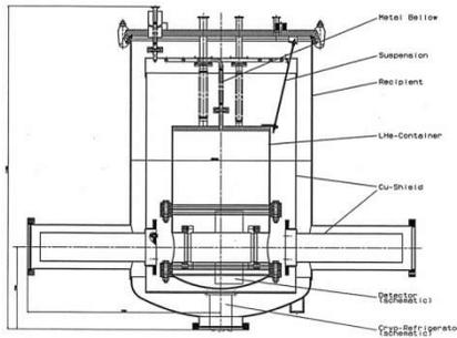
Figure 3: Cross section of the special bath-cryostat for the CCC at GSI.
