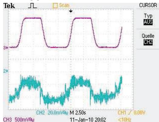
Figure 2: Dark current of about 5 nA measured with the CCC (lower curve) at “HOBICAT” (Helmholtz-Zentrum Berlin) compared with a reference signal of the accelerator voltage (upper curve).
