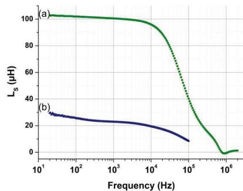
Figure 6: Frequency dependence of the inductance of the Nanoperm pick-up coil for FAIR (a) and VITROVAC 6025 F pick-up coil for DESY (b).
