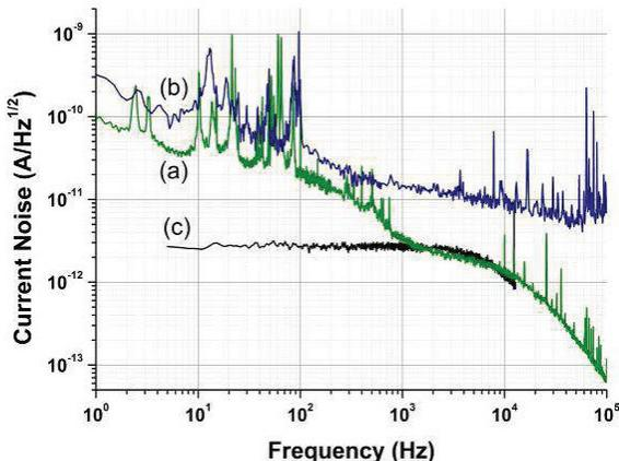
Figure 7: Current noise of the FAIR-CCC with Nanoperm M 764 core (a) in comparison with the DESY-CCC with VITROVAC 6025 F core. The intrinsic noise of the SQUID is depicted in curve (c).
