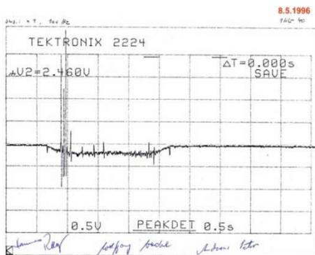
Figure 4: Worldwise first beam measurement of  $^{20}\text{Ne}^{10+}$  ions using a SQUID-based CCC at GSI.
