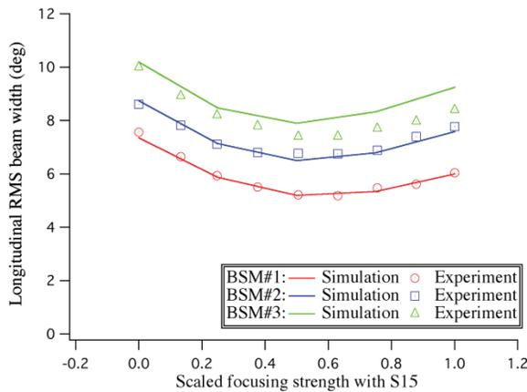
Figure 5: Measured longitudinal RMS beam width with changing focusing strength of last SDTL cavity (S15) and corresponding simulation results [5].
