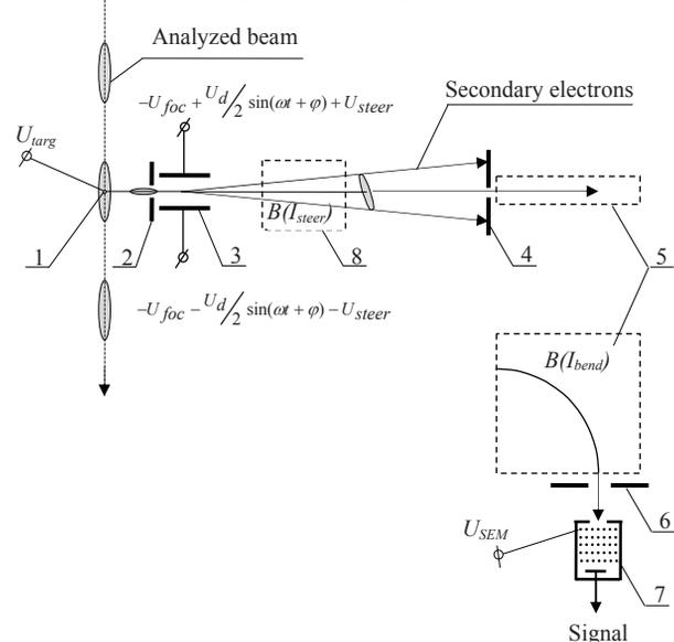
Figure 1: Principal of BSM (1: target, 2: input collimator, 3: RF deflector combined with electrostatic lens, 4: output collimator, 5: bending magnet, 6: collimator, 7: Secondary Electron Multiplier, 8: steering magnet)
