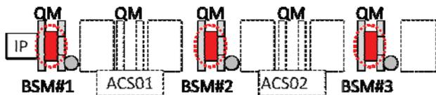
Figure 3: Bunch shape monitors (BSM) layout in the beginning of ACS section. Dotted circles are BSMs, QMs are quadrupole magnets (dotted QMs will be installed) and IP is an ion pump.
