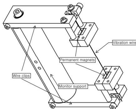
Figure 1: The VWM for beam halo measurement which was developed by Bergoz corporations [6].
