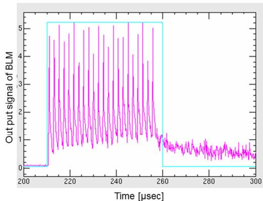
Figure 4: Output signal of the BLM at 1.3mm of distance from beam center.
