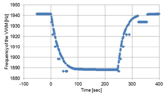
Figure 3: The VWM frequency shift at 1.3mm of distance from beam center. The wire was irradiated only in a period between 0 sec and 247 sec.
