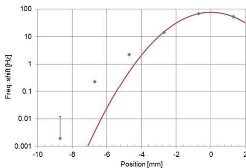
Figure 5: The result of the beam profile measurements for the scanning at the horizontal axis by the VWM.
