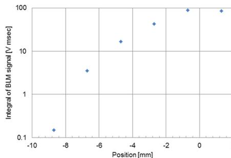
Figure 6: The result of beam profile measurements by integrated BLM signals at each the VWM position.
