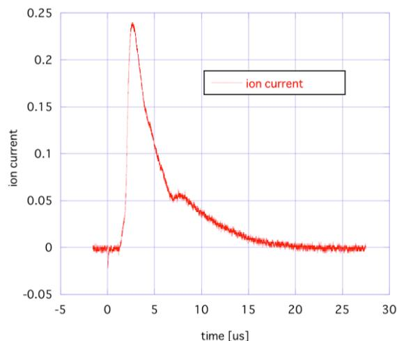
Figure 5: The ToF spectrum at detector position measured by a conventional Faraday cup in advance.
