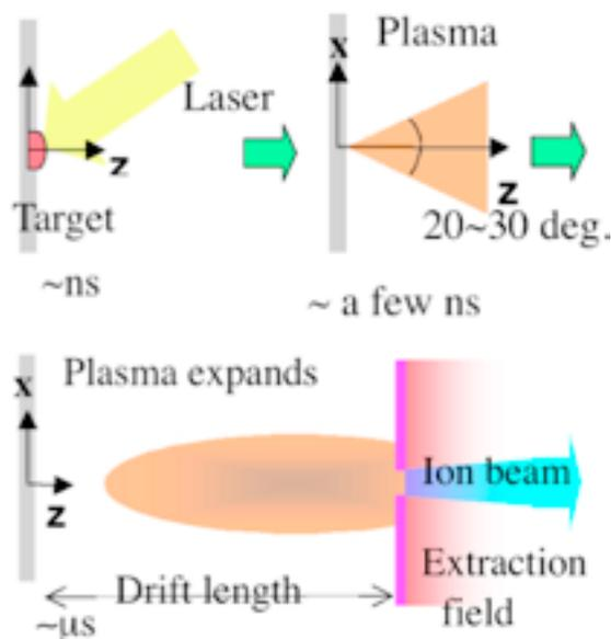
Figure 1: Image of DPIS (Direct Plasma Injection Scheme)
