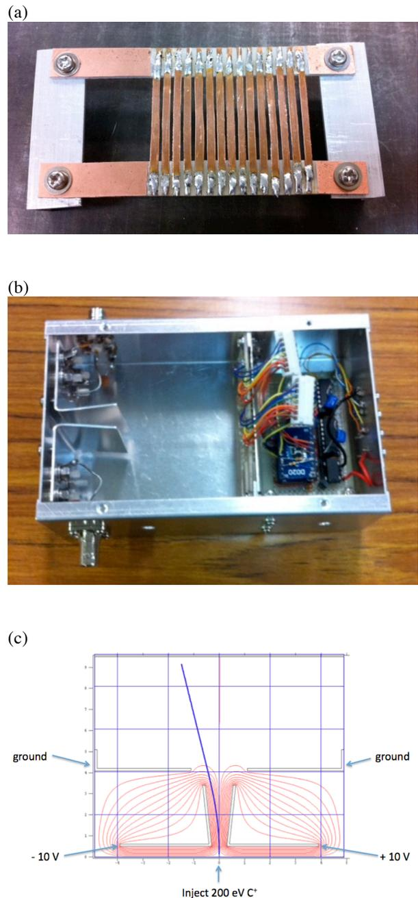
Figure 3: (a) multi-strip electrodes. (b) a picture of test model. (c) a deflector shape and the calculated orbit of 200 eV carbon (1+) ion deflected by electric field (deflecting electrode voltage is +/- 10 V).
