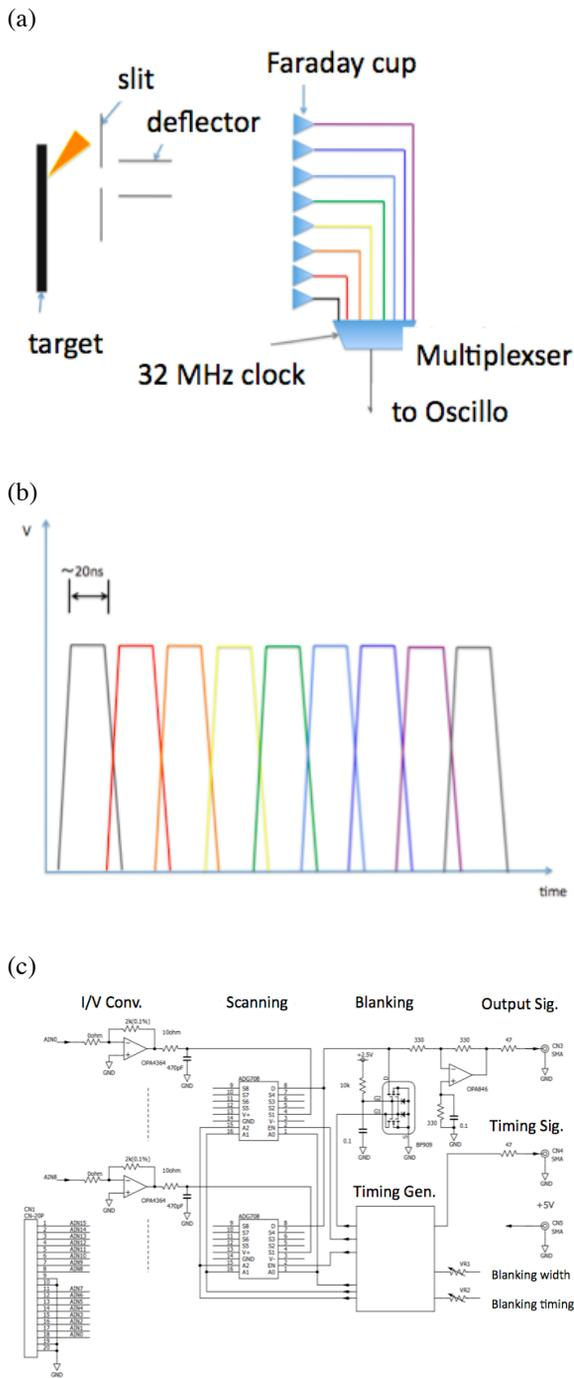
Figure 2: (a) a concept of our detector. (b) an image of multiplexing (the colors correspond to the line colors in (a) ). (c) the diagram of multiplexing readout circuit.
