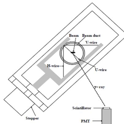
Figure 1: Structure of wire scanner [3].
