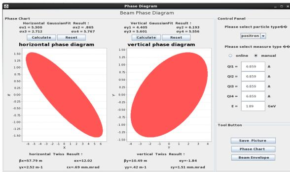
Figure 5: Emittance calculation.
