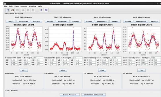
Figure 4: Beam size calculation.
