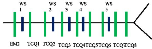
Figure 3: Wire scanners layout at the downstream of BEPCLII linac.
