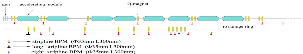
Figure 1: Schematic of the HLS II injector and of the BPM types built in.
