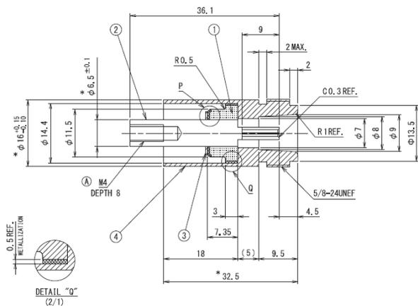
Figure 7: Special modified N type feed-through.
