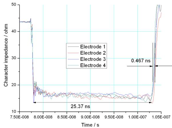
Figure 5: Impedance measurement results using the TDR (Time Domain Reflection) method.
