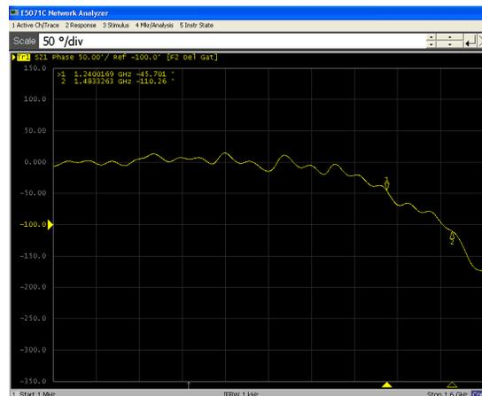
Figure 2: Phase dispersion measurement on a test bench.
