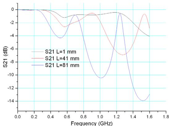
Figure 8: Transmission comparison from simulation for different length of the triangle section.
