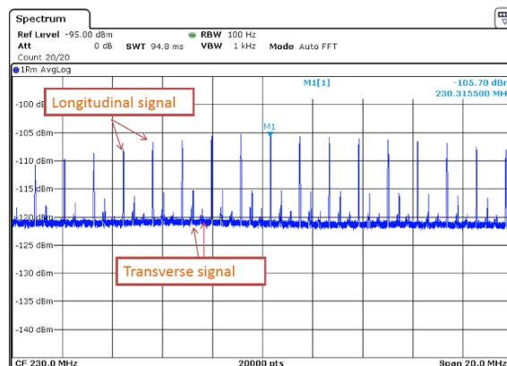
Figure 9: Beam measurement with the slotted pickup.
