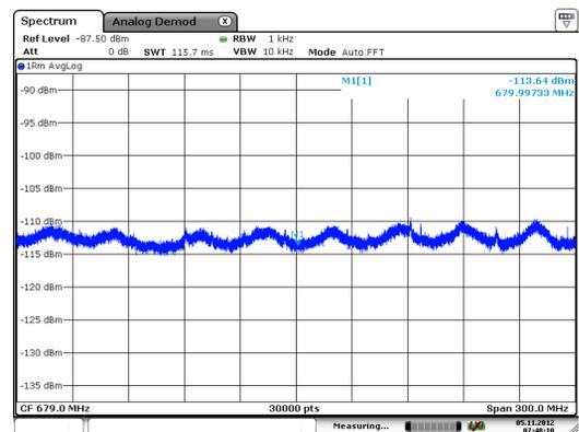
Figure 6: Noise measurement of the electrode.
