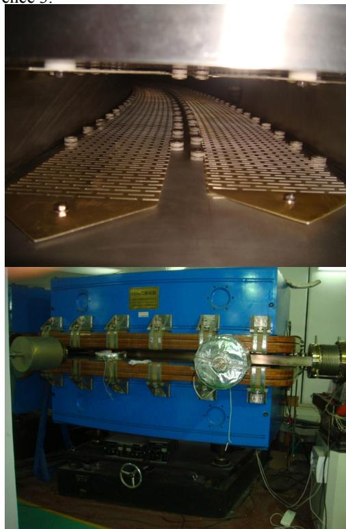
Figure 1: The slotted stripline electrode inside the bending vacuum tube (top) and the pickup tank installed on CSRe.
