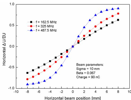
Figure 3: Simulation of the Difference over Sum method for CBPM for the fundamental, first and second harmonic frequency.
