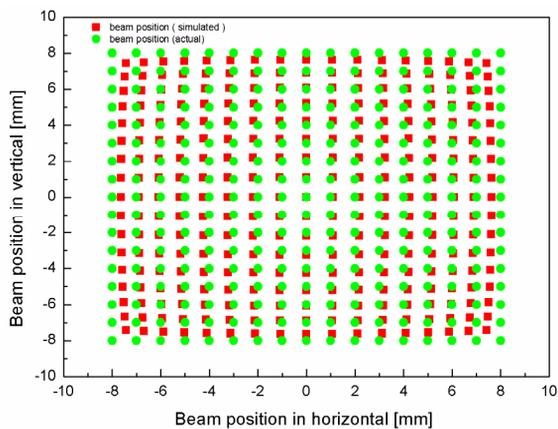
Figure 2: Sensitivity map of the CBPM at 162.5 MHz and  $\beta = 0.067$ .
