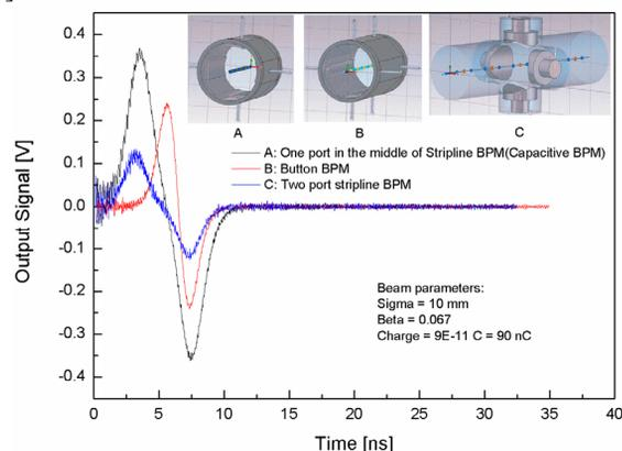
Figure 1: Comparison of the output signal from the different BPM models when the same parameters beam passing BPM.
