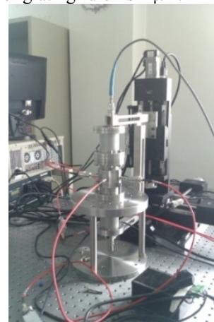
Figure 5: Photograph of ADS Injector II BPM test bench.
