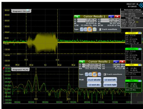
Figure 7: Output signal from CBPM on Proton LINAC in IHEP, CAS. The beam energy was 3.5MeV with bunch frequency of 352.2 MHz. The beam current was 15 mA with the macro bunch length of 50  $\mu$ s.
