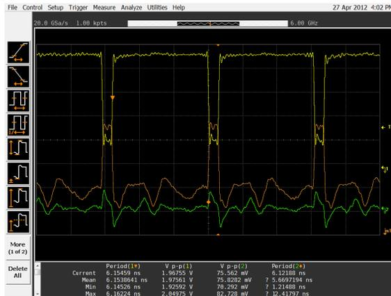
Figure 6: Output signal from CBPM on the test bench.
