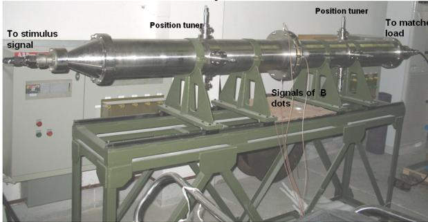
Figure 3: The coaxial test stand for the development of composed B dots monitors.
