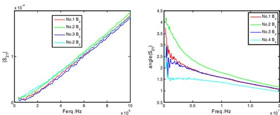
Figure 7: Signals of axial B dots when the tilt of the inner conductor is 16mrad in y direction.
