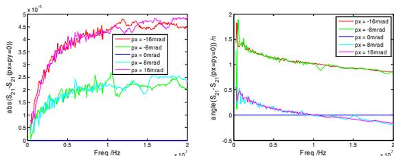
Figure 8: Signals of axial B dots at various transverse tilt.
