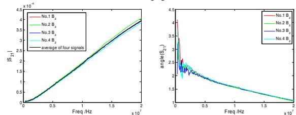
Figure 6: Signals of axial B dots when the inner conductor is on axis.
