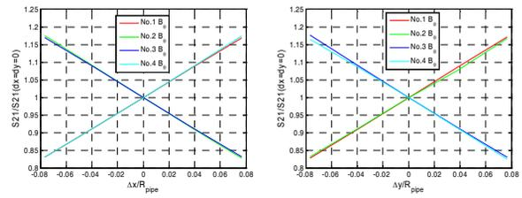
Figure 5: Ratio between the signal with transverse displacement and the signal on axis vs transverse displacement.
