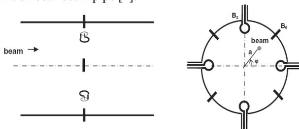
Figure 1: Azimuthal B dots and axial B dots are composed in a single device to measure beam current, displacement, and beam deflection angle.
