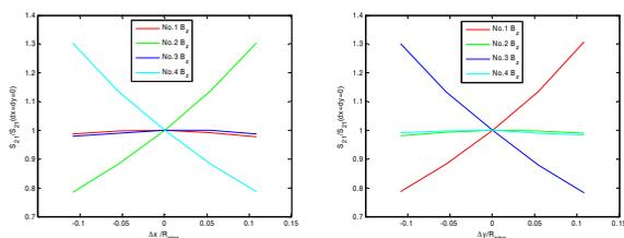
Figure 9: Response of the axial B dots to transverse offset.
