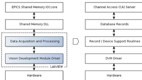
Figure 4: The block diagram of DCCT IOC.
