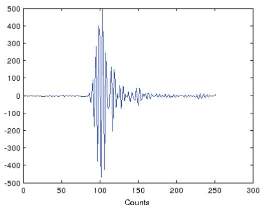
Figure 7: The BPM raw ADC signal.
