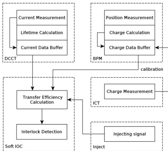
Figure 6: The block diagram of transfer efficiency measurement.
