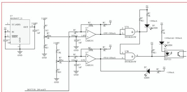
Figure 3: Beam current interlock module.
