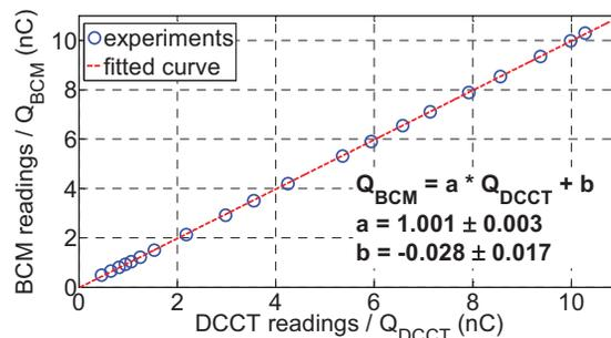
Figure 1: The linearity of beam charge measurement
