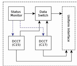
Figure 5: The DCCT redundancy architecture.
