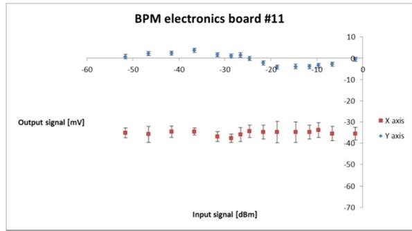
Figure 4: Measurement of the BPM electronics board signal reliability.
