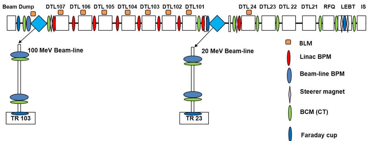
Figure 1: Layout of beam diagnostics in KOMAC 100-MeV linac and beam lines.
