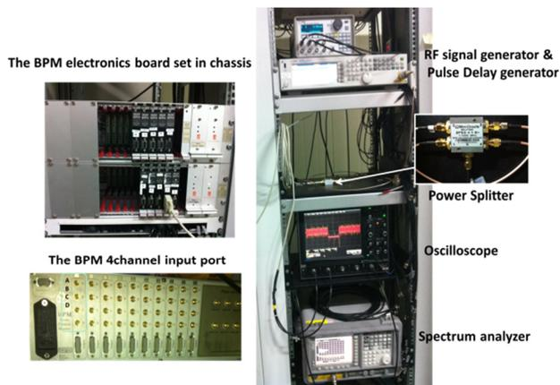
Figure 5: Photo of the set-up the electronics test.
