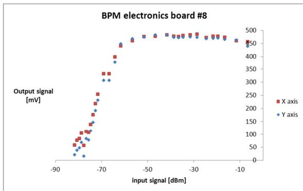
Figure 3: The result of the lowest measurable signal using the BPM electronics board.
