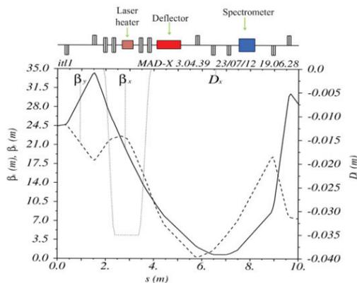
Figure 1: Lattice for PAL-XFEL Injector.
