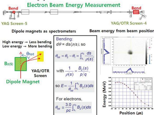
Figure 8: Electron beam energy measurement.
