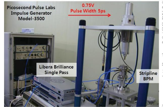
Figure 6: Stripline BPM and BPM Test-stand.
