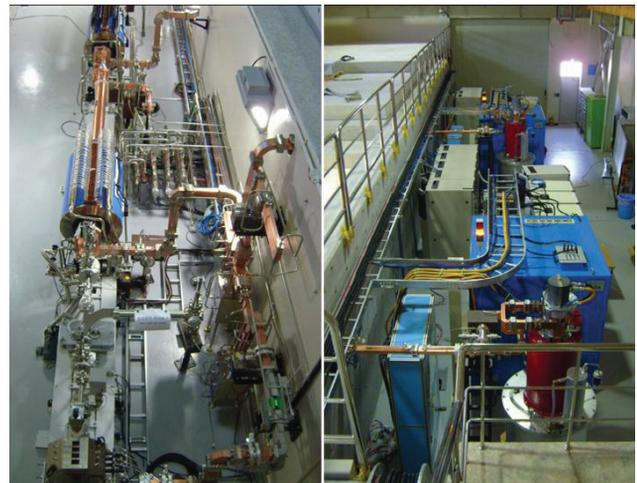
Figure 3: PAL-ITF. (left) Gun & Injector, (right) Klystron & Modulator.
