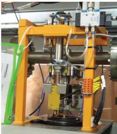
Figure 3: Beam flag at the booster ring
