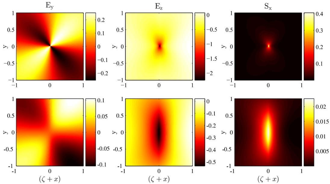
Figure 3: “Snapshots” of the wave field and the component  $S_x$  of the Poynting vector in the plane  $x=\text{const}>0$  for the point charge;  $a_0 = 0$  (first row) and  $a_0 = 0.5c/\omega_p$  (second row);  $\beta = 1$ ; electric field is in  $q\omega_p^2/c^2$  units;  $S_x$  is in  $q^2\omega_p^4/c^3$  units; coordinates in  $c/\omega_p$  units.
