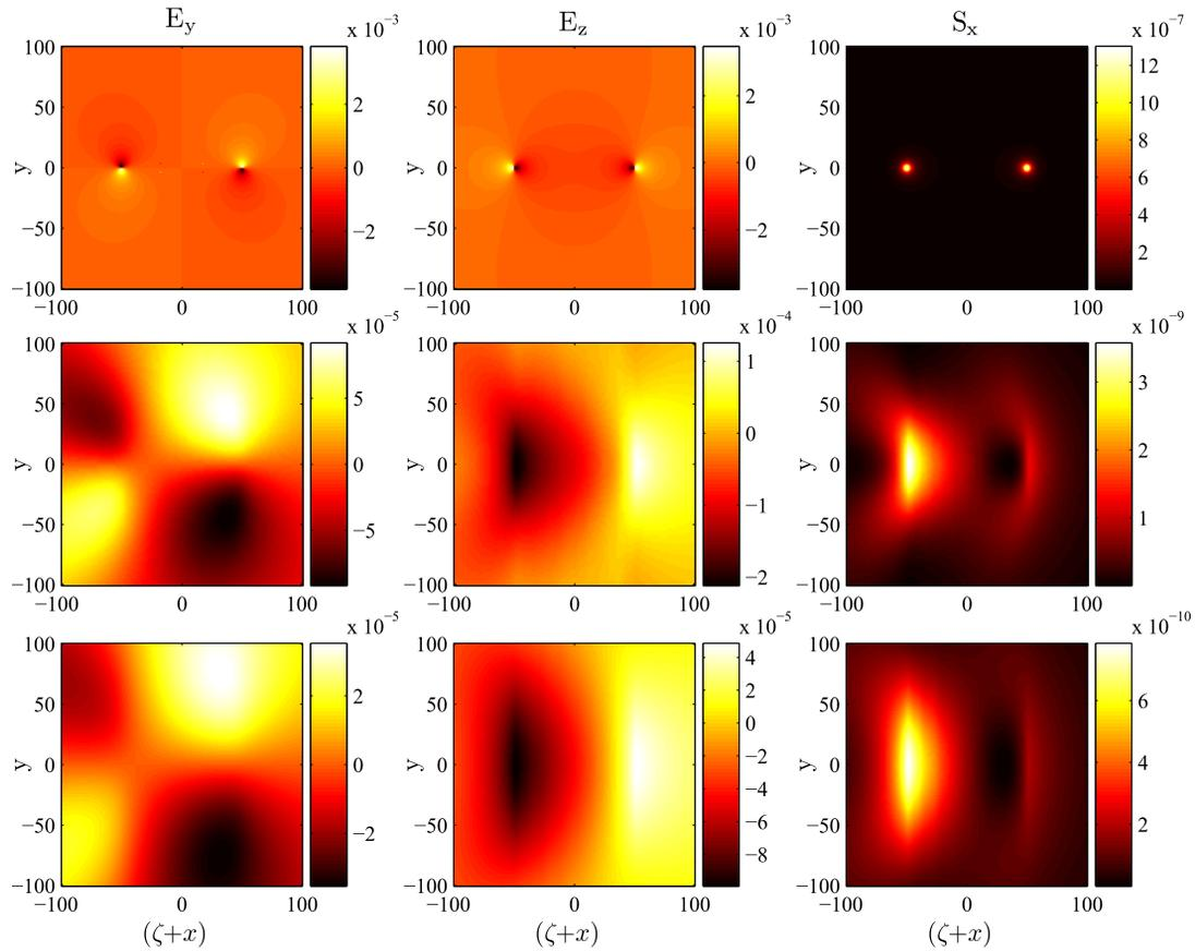
Figure 4: “Snapshots” of the wave field and the component  $S_x$  of the Poynting vector in the plane  $x=\text{const}>0$  for the linear bunch in the unbounded metamaterial (first row) as well as in the semi-bounded one for  $a_0 = 50$  (second row) and  $a_0 = 100c/\omega_p$  (third row);  $\sigma = 50c/\omega_p$ ;  $\beta = 1$ ; electric field is in  $q\omega_p^2/c^2$  units;  $S_x$  is in  $q^2\omega_p^4/c^3$  units; coordinates in  $c/\omega_p$  units.
