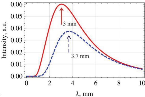
Figure 3: The calculated spectra of coherent DR from single plate of a target.
