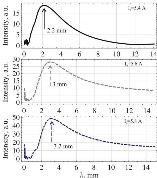
Figure 6: The reconstructed spectra from double DR target interferograms.
