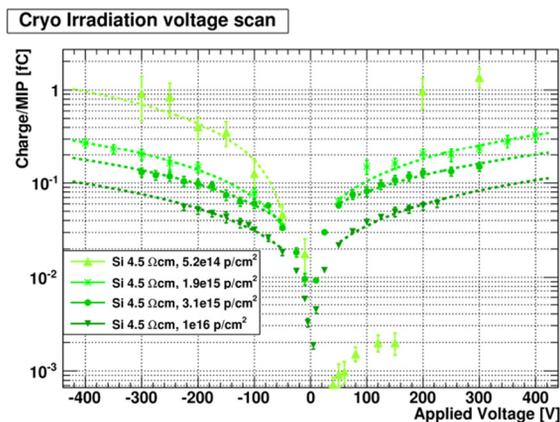
Figure 10: Voltage scan for 4.5  $\Omega\text{cm}$  silicon.
