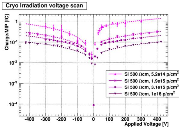
Figure 9: Voltage scan for 500  $\Omega\text{cm}$  silicon.
