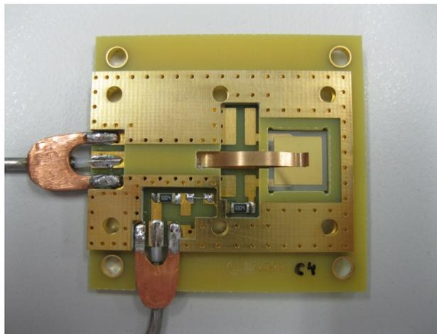
Figure 3: Holder for DC readout from Cividec.
