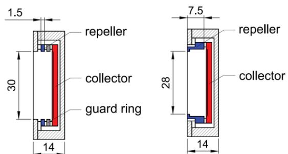
Figure 2: Layout of the prototype Faraday cups. Dimensions in mm. Left: Prototype 1. Right: Prototype 2.
