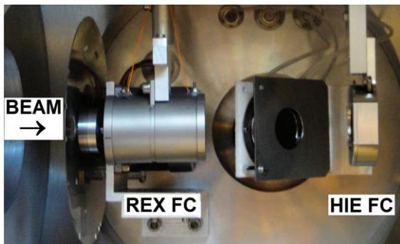
Figure 3: Experimental setup. The short prototype ( HIE) FC was installed in a diagnostic box, which also includes a collimator wheel and a standard (REX) FC.
