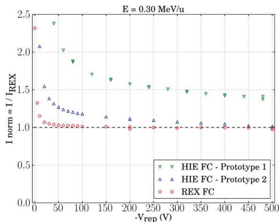
Figure 5: Normalized current as a function of the repeller potential for ions with energy  $E = 0.30$  MeV/u.
