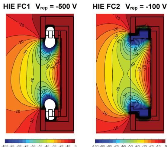
Figure 4: Electrostatic potential inside the HIE FC (V). Left: Prototype 1, biasing the repeller to -500 V. Right: Prototype 2, biasing the repeller to -100 V.
