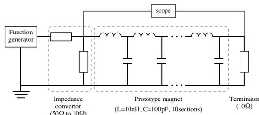
Figure 6: Measurement system.
