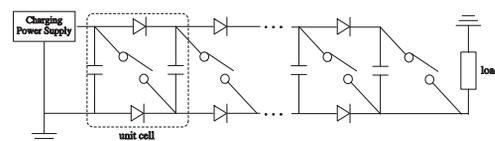
Figure 2: Simplified diagram of a Marx cell.
