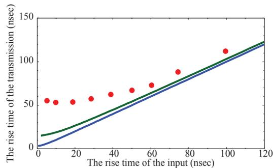
Figure 8: Dependence of transmission rise time for input rise time. Measured data is shown as dots (red), simulated data is shown as line (blue, green).
