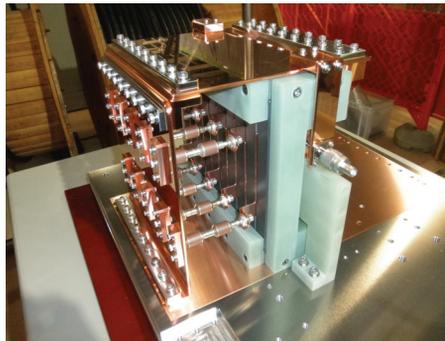
Figure 5: Photograph of the prototype kicker.
