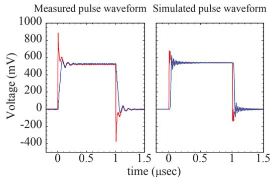
Figure 7: Comparisons with measured (left) and Simulated (right) waveforms. Red line is input and blue line is transmission signal in both plots.
