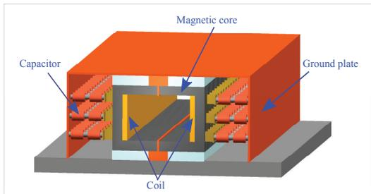
Figure 4: The conceptual design of compensation kicker magnet.
