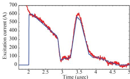
Figure 3: Real tail field (red) and the Waveform reproduced on the simulation (blue).
