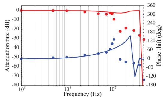
Figure 9: Comparisons with measured (dots) and simulated (solid lines) frequency characteristics. Red is the attenuation rate (right axis) and blue is phase shift (left axis) in both plots.
