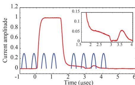
Figure 1: At 4th injection timing, the position relation between the injection kicker's excitation current (red) and beams (blue). Upper right is extended figure of the tail field. The current waveform is normalized by flat top value.
