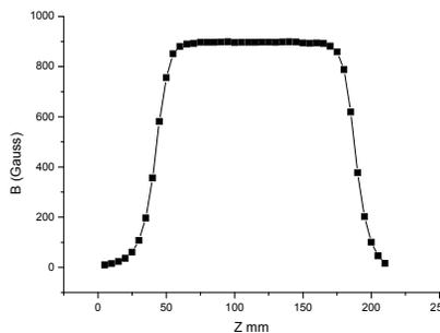
Figure 11: Field profile along z-axis of the of kicker.
