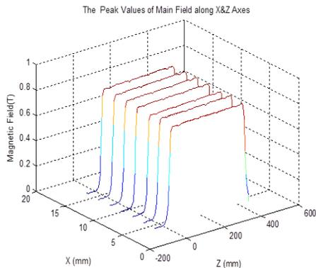
Figure 10: Field profile along z-axis of the septum magnet.
