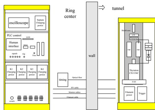
Figure 7: Pulsed power control.
